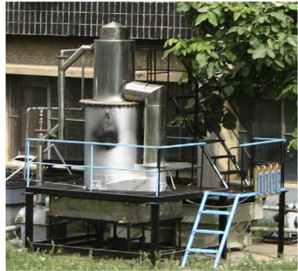
Fig. 9. A view of 75 kWth, downdraft biomass gasifier.
